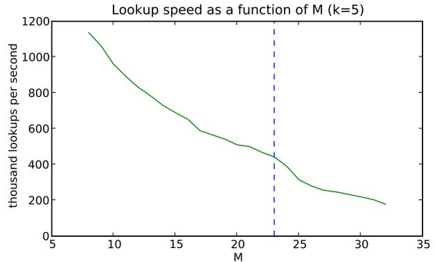
**Figure 2. Increasing the size of the Bloom filter decreases its speed due to caching issues. The dashed line indicates the 2 MB (8 Mbit) size of the benchmark system’s L2 cache. (Note: these speeds are for successful lookups; the speed of looking up hash values not in the filter are roughly 12× faster.)**
